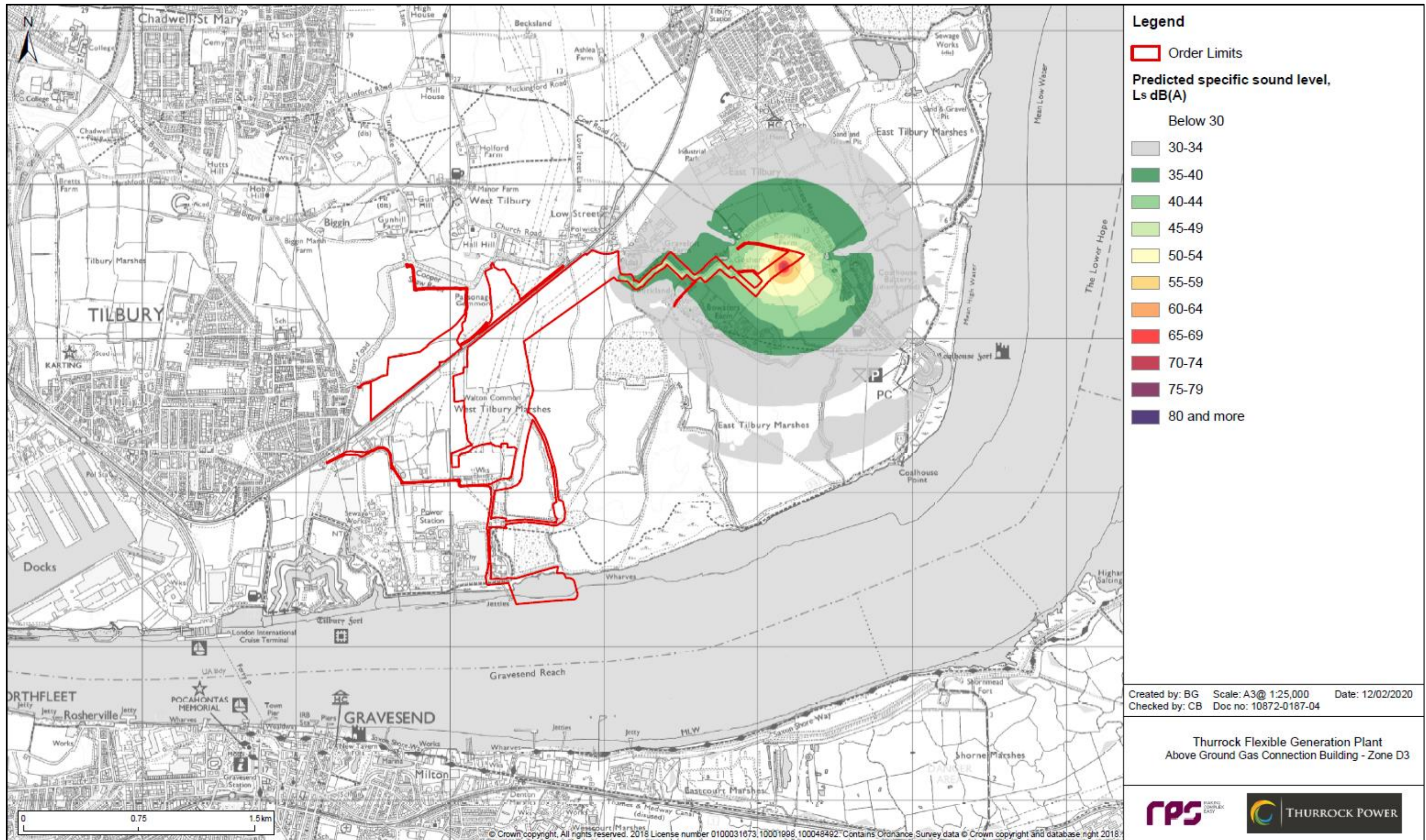
Figure 4.14: Construction – Construction of Above Ground Gas Connection Building.
