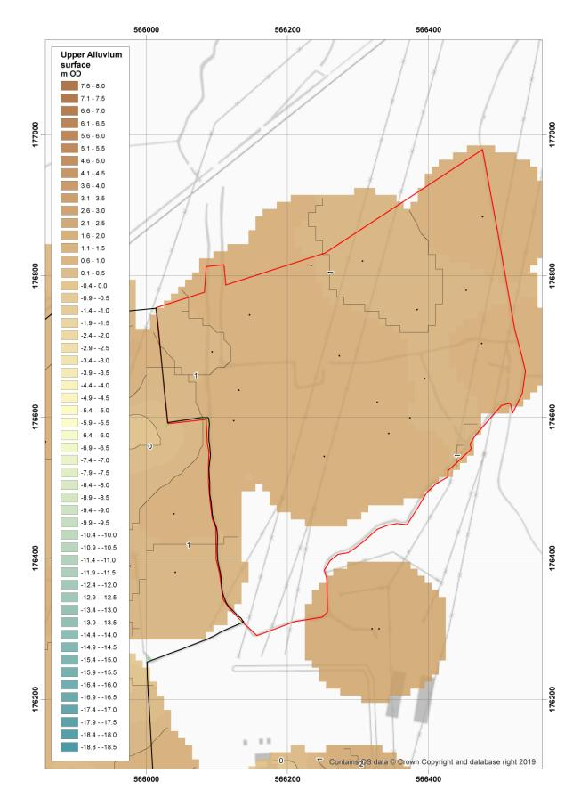
Figure 19: Surface of the Upper Alluvium (m)
