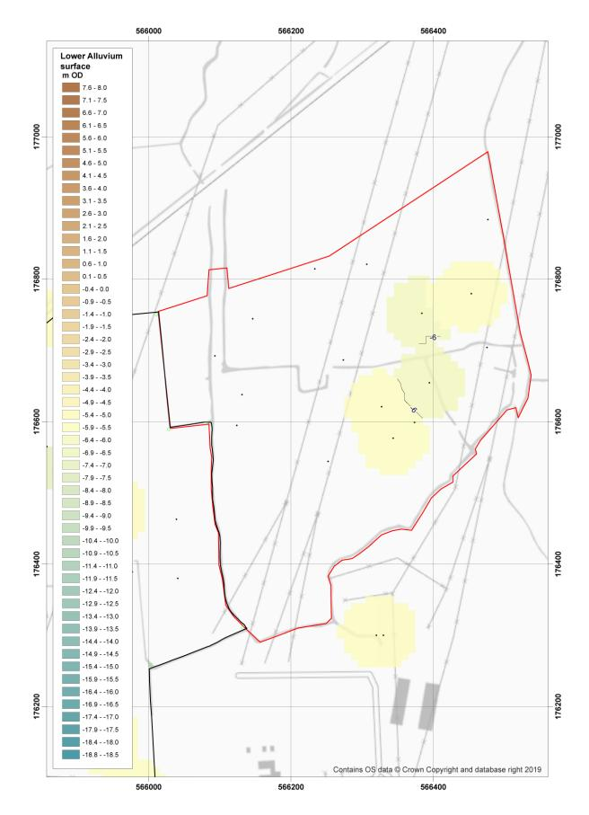
Figure 9: Surface of the Lower Alluvium (m OD)
