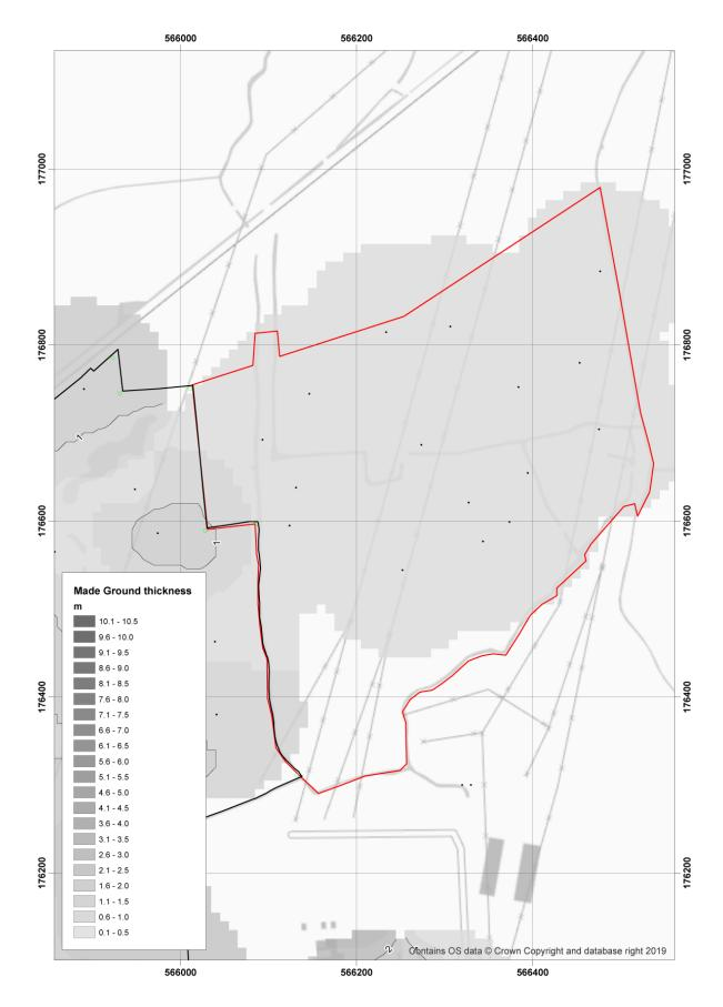
Figure 23: Thickness of Made Ground (m)
