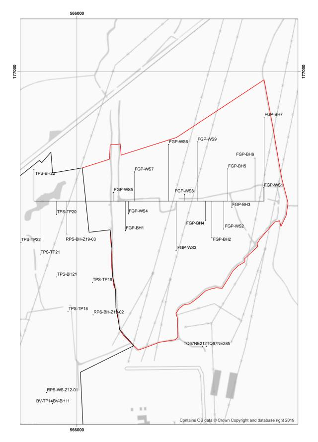
Figure 3: Location of geotechnical site investigations (cable percussion boreholes and window samples only)
