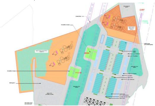
Figure 4: Indicative carbon capture layout
