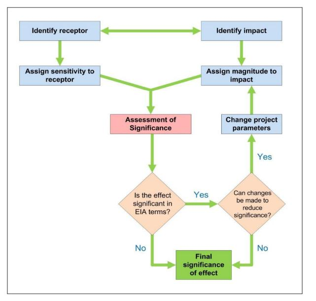
Figure 2.1: Iterative approach to measures adopted as part of the project within the Thurrock Flexible **Generation Plant**
