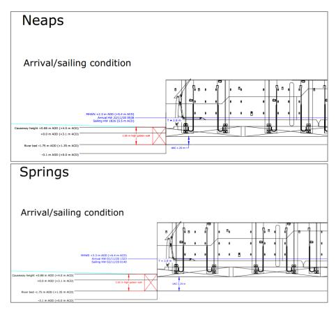
Figure 13: Terra Marique position relevant to Causeway at MHWN and MHWS
