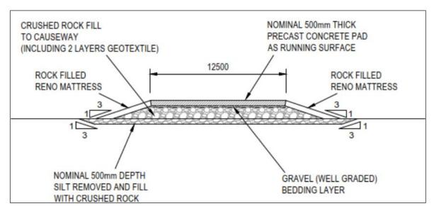
Figure 14: A typical Cross Section of the Causeway
