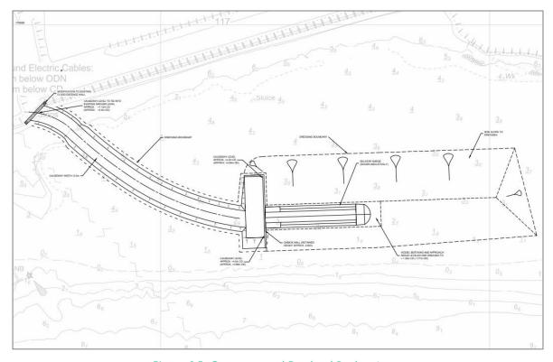
Figure 15: Causeway and Dredged Pocket Area.
